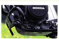
Engine guard and skidplate help protect the engine cases from expensive damage caused by falls or impacts when riding over rugged, rocky terrain.
