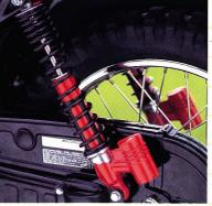
New remote reservoir shocks work with the long-travel rear suspension to give extra riding comfort when the going gets rough, and the loads heavy. Spring preload adjuster lets you select the right suspension setting for the job. Long-stroke front suspension gives compliant ride and assured handling.
