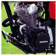
Rugged Honda 4-stroke engine gives you big power when you need it. Quiet, economical, and reliable OHC powerplant features a no-maintenance CDI. Versatile 5-speed auto-clutch transmission gets you moving with a minimum of bother.
